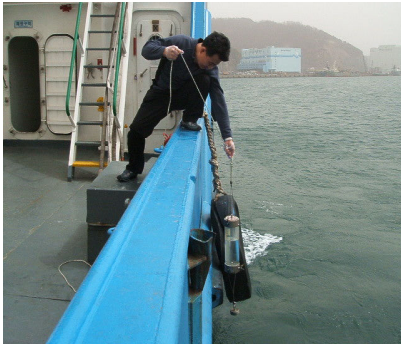
Fig. 5. Sampling seawater by water sampler
