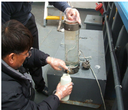
Fig. 6. Transportation of sampled seawater from sampler to bottle
