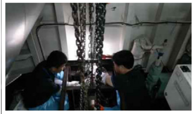
No.1 축계 Support Bearing 조립
